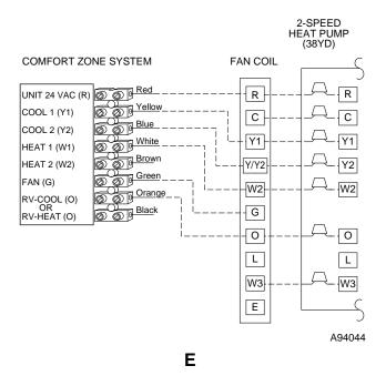
Fig. 21—Typical Wiring Diagrams (Fan Coil with Heat Pump) Continued
